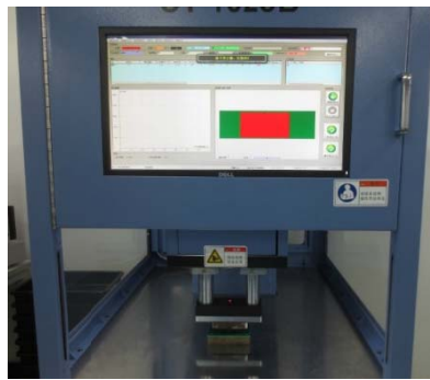
d) The module is pressed into the PCB with the stated force. e) After the assembly the Push-pull force tester monitors the total force.
