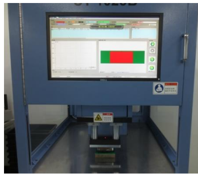
e) After the assembly the Push-pull force tester monitors the total force.
